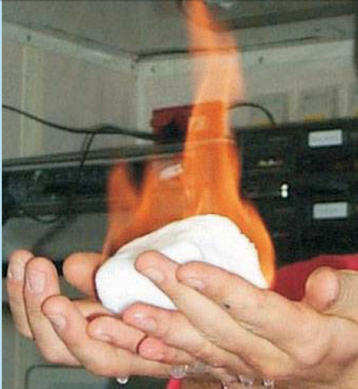
Figure 2. Fire and ice. A chunk of methane clathrate displays its potential as an energy source. As the compound melts, released gas feeds the flame and the ice framework drips off as liquid water. (Courtesy of Gary Klinkhammer, Oregon State University.)
