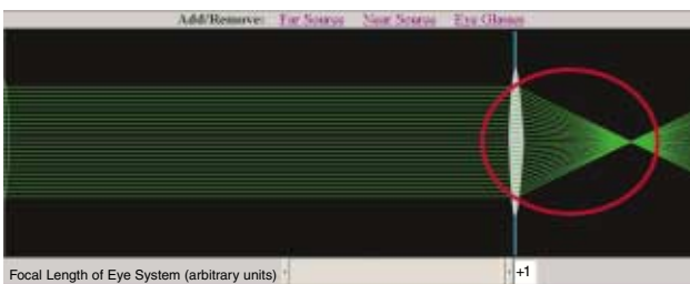
Fig. 5(a). Light from very far away is focused in front of the retina.
